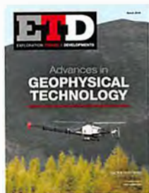
Cover photo: Flying-Cam's SARAH e 4.0 unmanned helicopter, equipped with a Scintrex CS-VL cesium-vapour magnetic sensor and RMS Instruments' AARC51 adaptive aeromagnetic real-time compensator, in flight near Chifeng, Inner Mongolia, China. Credit: Flying-Cam
